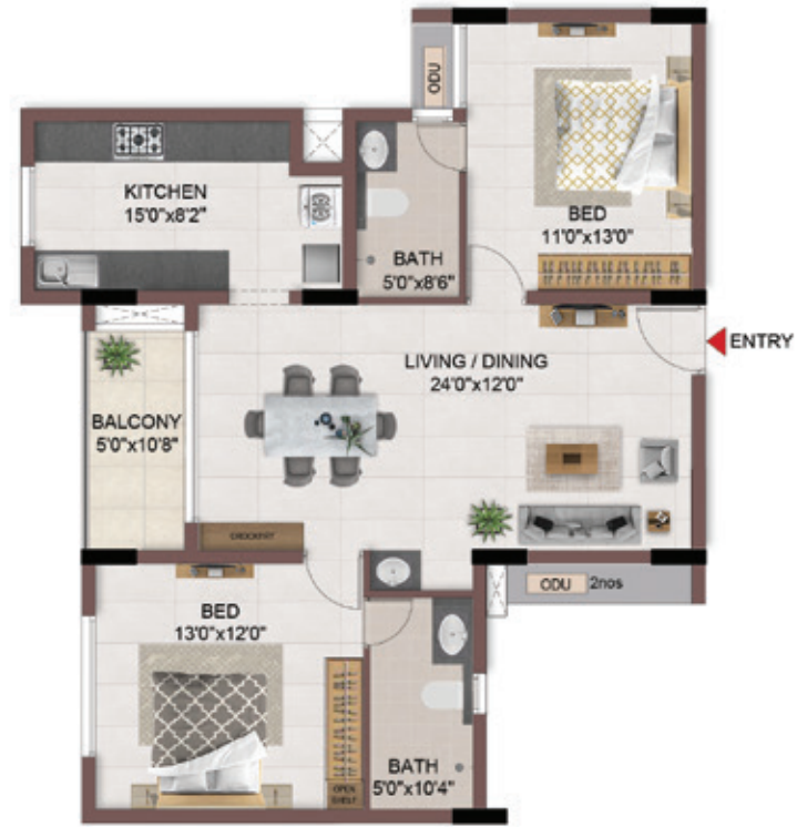
TYPICAL FLOOR 1ST TO 5TH
