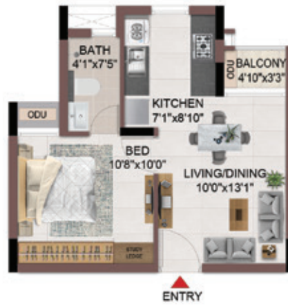
TYPICAL FLOOR 1ST TO 5TH
