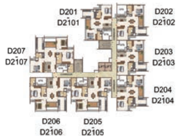
BLOCK 4 & 5 TYPICAL FLOOR PLAN ( 2ND TO 21TH )
